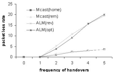
Packet drop rates for ALM and IP multicast [f1]
