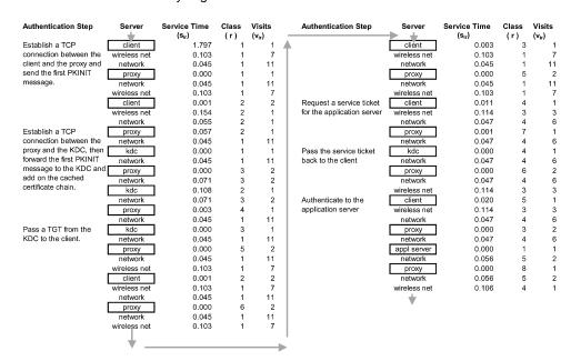
Fig. B.1. The MP-PKINIT transaction and its modeling parameters.
