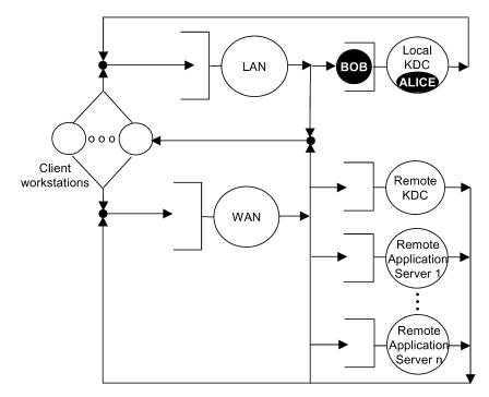
Fig. 1. Modeling topology for a multiple-realm authentication.
