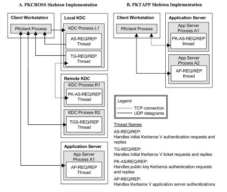
Fig. 3. The public-key-enabled Kerberos skeleton software architecture.
