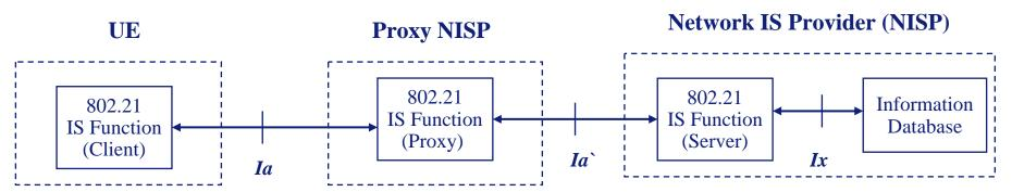
Ia: Interface between UE and Network IS providerIx: Interface between IS function and Information Database
