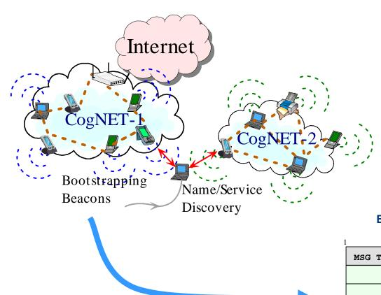
Establish network connectivity after a cognitive radio device is turned on or enters a new service area
